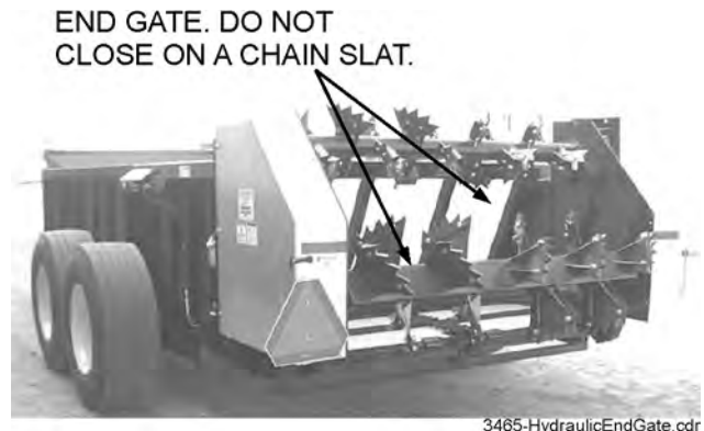
FIGURE 9. HYDRAULIC END GATE, VIEW FROM REAR
