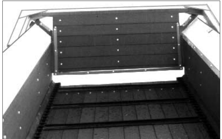
FIGURE 5. OPTIONAL HYDRAULIC END GATE, CLOSED
